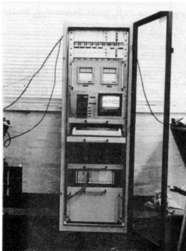
Figure 4. Arrangement of Data Logging System for Full Scale Evaporator Rig.
