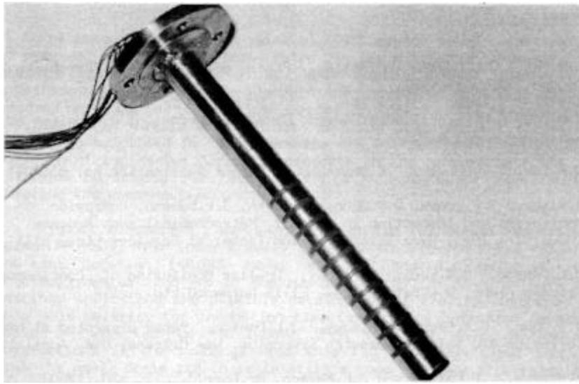
Figure 1. General Multi-element Electrochemical Probe Arrangement.
