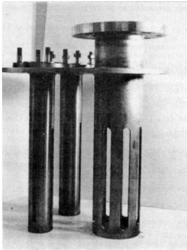
Figure 2. Probe Shield Arrangement on the Full Scale Test Rig.
