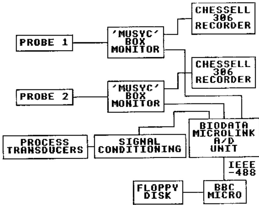
Figure 5a. Block Diagram of the Full Scale Evaporator Monitoring System.
