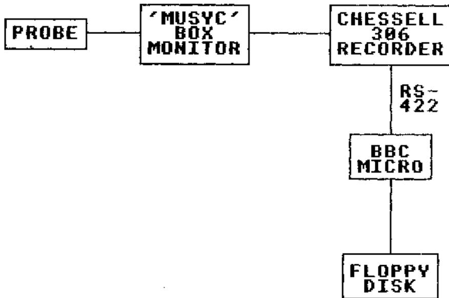
Figure 5b. Block Diagram of the Laboratory Rig Monitoring System.
