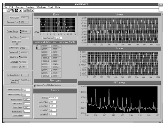
FIGURE 7. Layout of the computer interface for the harmonic and intermodulation measurements with a programmable potentiostat.
